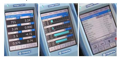
The Intelligent Viewer (I-Viewer) is an application software run on the PC to analyze, store and print out the ECU data captured by the Intelligent Tester II. The data files stored in the I-Viewer can be transferred by attaching to an e-mail. Software Update Wizard and Calibration Update Wizard of ECU reprogramming will be a function of the I-Viewer.
